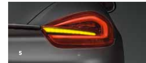
1 Night design, front 2 Night design, rear 3 Taillight 4 Brake light 5 Taillight and direction indicator
